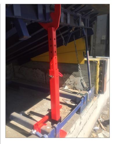
Shown on a CentraAir Series dock leveler, the Tough Strut will help provide safety at the loading dock by adding another means for additional support to air or mechanical levelers during maintenance.
